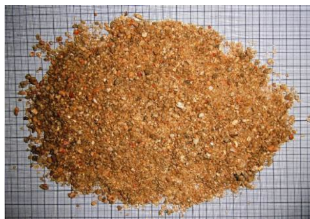
Figure 8. Example of filter material used for VFBs for municipal wastewater treatment in Brazil: coarse sand from river, containing neither loam nor silt (photo by C. Platzer, 2008).
