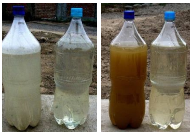
Figure 4. Wastewater samples before and after treatment in a VFB. Left photo: pre-treated greywater (left bottle) and effluent of the CW which is reused for irrigation of crops (right bottle). Right photo: pre-treated blackwater (left bottle) and effluent of the CW which has the typical brownish colouration caused by humic acid (right bottle) (photos by: H. Hoffmann, 2008).
